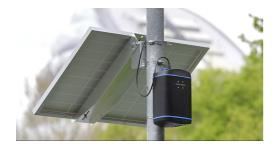
A real time Mcerts dust monitor can accurately measure low levels of pm10, pm2.5 and pm1
