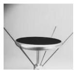
Frisbee-type dust deposit gauges are widely used in the UK for passive dust monitoring, especially during construction and industrial activities
